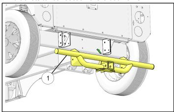
5. Reinstall bed support bolts and nuts as shown. The bumper ① should now hold itself in place. Torque bolts to specification.
