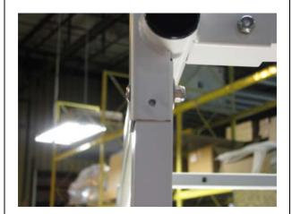
• Lift the ladder rack in to position.
