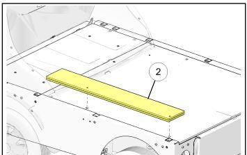
3. Insert lock and work adapter ① into bed location as shown. Lock in place with detent pin ⑨.
