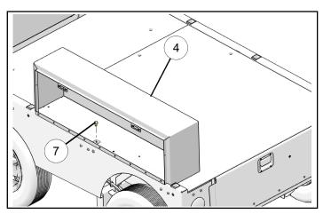
5. Insert remaining two bolts (§) in open holes, and torque to below specification.
