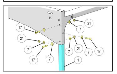
Slide four roll-in T-nuts <sup>(2)</sup> into OPS (2 per side) and attach OPS support bracket <sup>(1)</sup> with bolts <sup>(1)</sup> and washers <sup>(2)</sup> positioning the support brackets 15mm from the end of the OPS. Torque to specification.
