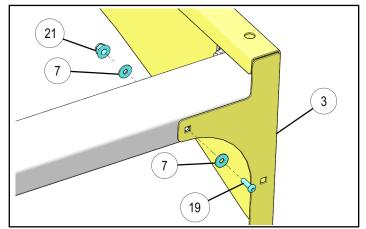
4. Attach the front tube ④ at both sides with bolts ⑱, washers ⑦, and nuts ⑳. Torque to specification.
