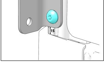
10. Attach ladder rack assembly to bed, by sliding in rear tubes into chassis as shown. Secure front tubes to OPS bracket (1) with bolts (18), washers (7), spacers (8), and nuts (2). Torque to specification.
