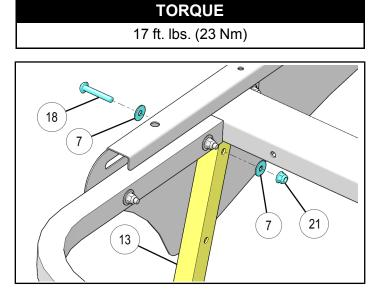
6. Attach LH and RH support brackets (5) (6) to front support tube with bolts (7), washers (7), and nuts
