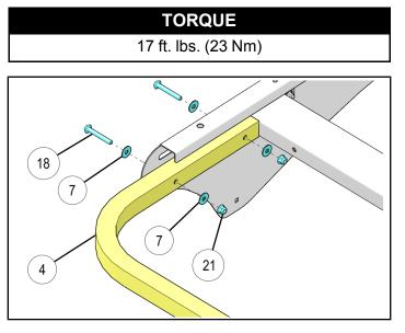
5. Attach front support tube (1) one on each side with bolts (1), washers (7), and nuts (2). Torque to specification.
