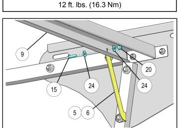
Attach rear tubes ① one on each side with bolts
