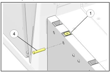
3. Final installation of front panel assembly as shown.
