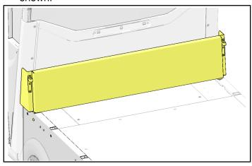
2. Mount front panel ② on bed using two screws ③ as shown. Torque to specification.
