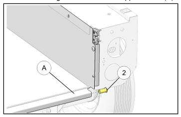
4. Attach tailgate assembly ① to bed with pivot pins
