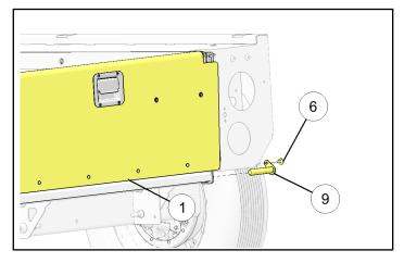
5. Final installation of hinged/ramped tailgate assembly is as shown below.
