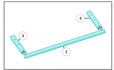
3. Loosely install screws (18) through washers (9) into tubes (4). **Do not tighten screws.**
