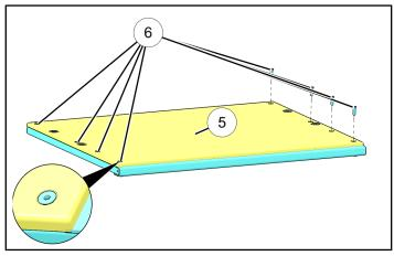
6. Keeping assembly flat, set in place on vehicle. Install four screws ① through tie-downs ② as shown. Torque screws to specification.
