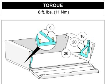
10. Loosely install two bolts (1) and two washers (26), and two nuts (24) into brackets (9) and (10) as shown. **Do not tighten bolts.**
