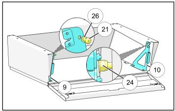
11. Close tailgate and adjust box to desired width. Counter-hold nut (2) and torque bolts (2) to specification.
