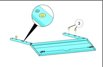
6. Place panel <sup>(1)</sup> into sides assembly ensuring holes line up through entire assembly.
