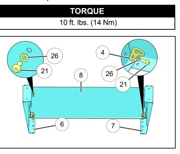
Set tailgate assembly flat and insert four spacers
