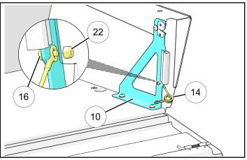
15. Attach other end of cables (4) to inside of tailgate lid bolt holes using bolts (6) and nuts (2) as shown. **Do not tighten bolts at this time.**
