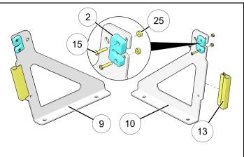
Bolt assembled brackets to the base using two bolts (2) and two washers (2). Torque bolts to specification.
