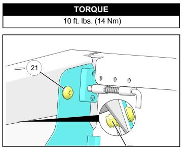
12. Adjust latch height, centering pin in latch , counterhold nuts (3) and hand tighten screws (15).
