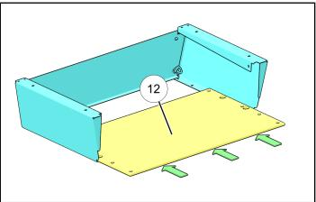
Set upper assembly onto tailgate assembly ensuring bolt holes line up. Install four rear screws
