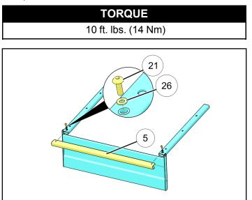
Attach side elements (6) and (7) to back element (8) by installing screws (2) through washers (26) on upper nut inserts and through washer (26) and tie-down bracket (4) on lower nut inserts. Torque screws to specification.
