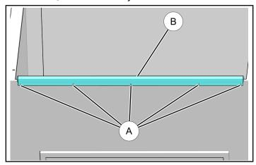
ii. Clean surfaces and install sealing tape (6) on base surface of each side panel as shown. Install bulb seal (7) to front bottom edge of box as shown.
