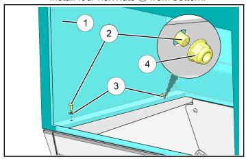
ii. Align short box ①. Counter hold 4 hex nuts④ and torque screws to specification.
