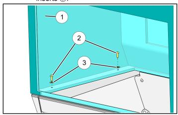
ii. Align short box ① and torque four screws②to specification.
