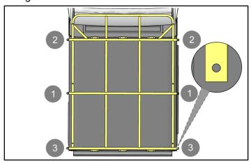
5. Install twelve screws ③ into holes in angle brackets ⑧. Tighten screws in sequence on each end as shown. Ensure brackets do not deform when tightened.
