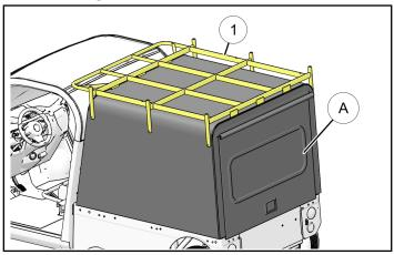
3. Center rack ① by aligning inner surface of angle brackets ③ with inner edge of rubber seal ⑥.
