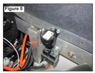
6. Determine location of mounting holes and mark with a pencil. Secure the beeper with the two provided self drilling screws (PN 7519456).
