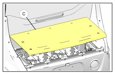
b. For eL XD: Remove six socket head screws (D) and three screws (E) using 5mm socket and ratchet to remove rear battery access cover (C).
