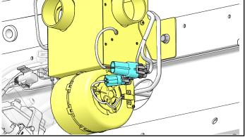
17. Install upper ① and lower ② heater vent ducts into blower box ③ and zip tie ⑦ as shown.
