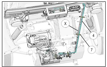
14. Finish routing the harness ④ under the front dash and zip tie ⑦ in the shown locations. Attach the heater harness to the accessory block (Y) by using 8mm socket and ratchet. Ensure the harness routing does not interfere with the vehicle steering.
