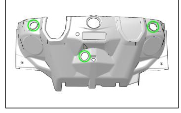
10. Cut out hole for heater switch installation in the upper dash panel using jig saw or dremel. This switch location is on left side of the interior light switch as shown.
