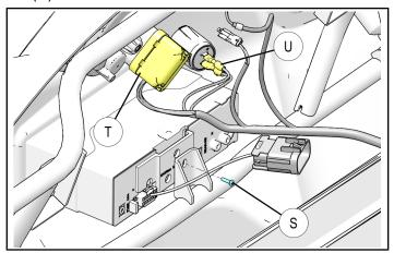
9. Cut out three holes in the lower dash panel for heater ports installation in marked area (highlighted in yellow) using template provided at the end of the instructions. Align template as shown on lower dash panel. Use jig saw or hole saw or dremel for cutting holes.
