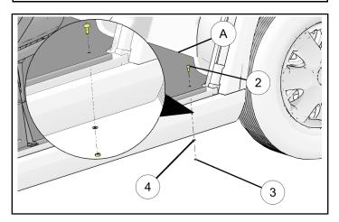
4. Install floor mats ① and ③ on floor (A) and secure by engaging the snaps studs installed in Step 3.
