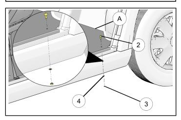
4. Install floor mats ① and ⑤ on floor (A) and secure by engaging the snaps studs installed in Step 3.
