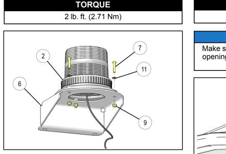
2. Slide two roll in T-nuts (1) into the OPS and attach the beacon light bracket (6) to the roll in nuts in the OPS with bolts (8), nuts (12) as shown.
