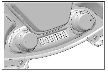
Attach the beacon light switch ④ to the upper dash lid. Connect the harness ③ to the switch ④ as shown.
