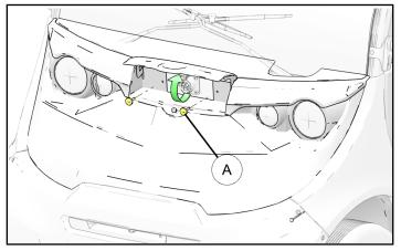
4. Remove the upper dash panel by loosening eight Tuflok <sup>®</sup> rivets (B) as shown.
