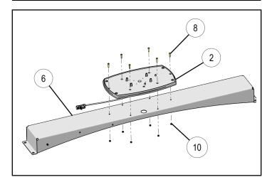
3. Reattach lens that was removed with four screws.
