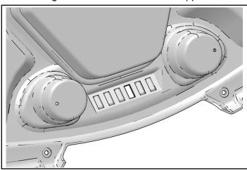
9. Attach the roof light switch ④ to the upper dash lid. Connect the harness ③ to the switch ④ as shown.
