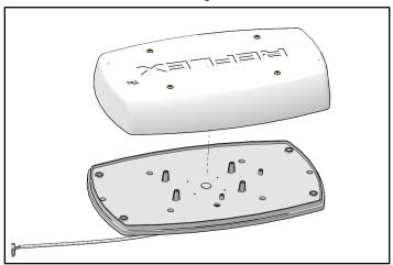
2. Attach amber light bar ② to mounting bracket ⑥ with six screws ⑧ and nuts ⑩.
