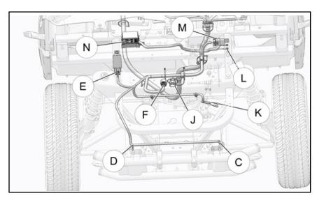
16. Tie the harness using panduit straps (11) at the shown locations to avoid contact with rotating parts and sharp edges and push the fastening clips into the corresponding holes in frame as shown in figure.
