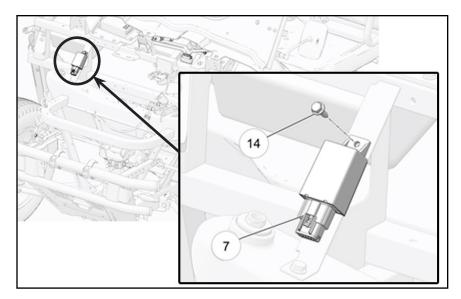
14. Install fuse block bracket (19) using two M6 screws (14) as shown in figure.
