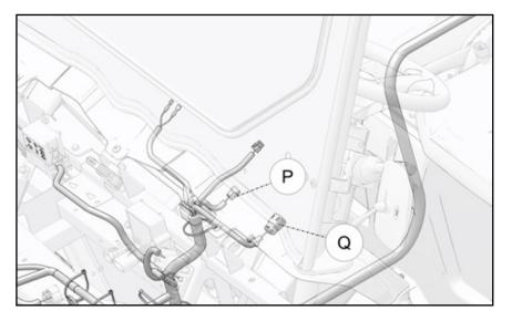
18. Route the parasite harness (2) under the vehicle body as shown path, Tie the harness to the main harness using panduit straps (11) at the shown locations to avoid contact with rotating parts and sharp edges.
