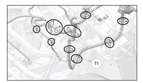
17. Make connections of the parasite harness (2) on the dash panel side as shown in figure.
