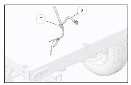
21. Make connections of the cargo box harness (3) with parasite harness (2) on the rear side of the vehicle and push the fastening clips into the corresponding holes in frame which are circled in the figure.
