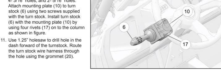
12. Cut 33.0 X 9.6 mm rectangular slot using a utility knife and snap turn indicator (4) in the dash panel (B) as shown in figure.
