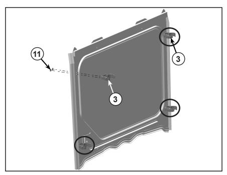
2. Install two half snap clamps (6) in the top mount locations of the windshield using four torx screws (11). See figure. Torque to 30 in-lbs. (3.4 Nm).
