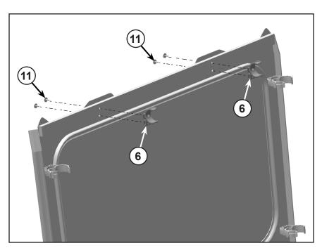
3. Align the assembled windshield (A) with the front cab frame of the vehicle. Once all clamps have been aligned with the frame bars, press down to each clamp to snap into place. See figure.
