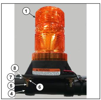
5. Connect the lamp with the wire terminal ring (2). Route the wire along with the ROPS bars as shown in the Figure and secure the routing with panduit straps (3).
