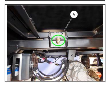
2. Install the shock ⑤ to hold the bed up. Engage the clevis pins ⑩ and hitch pin ⑨ clips with the shock as shown.
