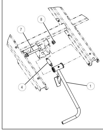
6. Install manual dump box on vehicle as shown.
