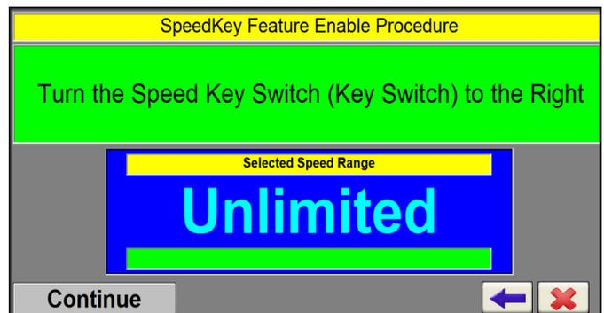
22. Speed Key Functionality is now installed. The feature can be uninstalled at any time by following Steps 1-6, but selecting the “Disable Speed Key Function” button. If the feature is deactivated for any reason, a new speed key kit will need to be purchased to re-install.
