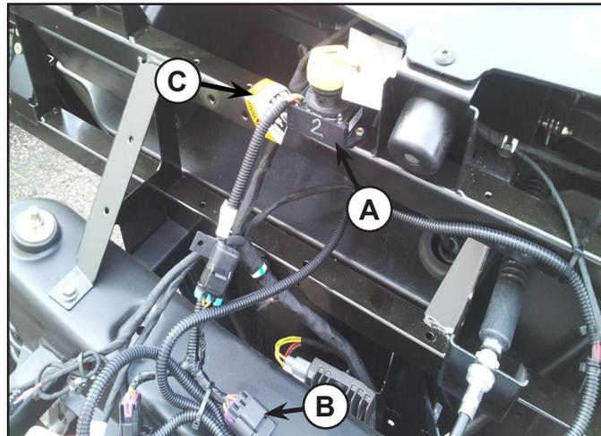
4. Locate the speed key module on cab support as shown in figure.
