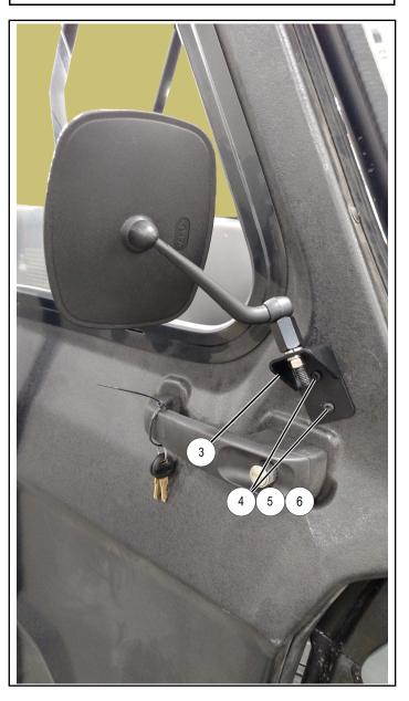
2. Assemble mirror to bracket using mount adapter.
