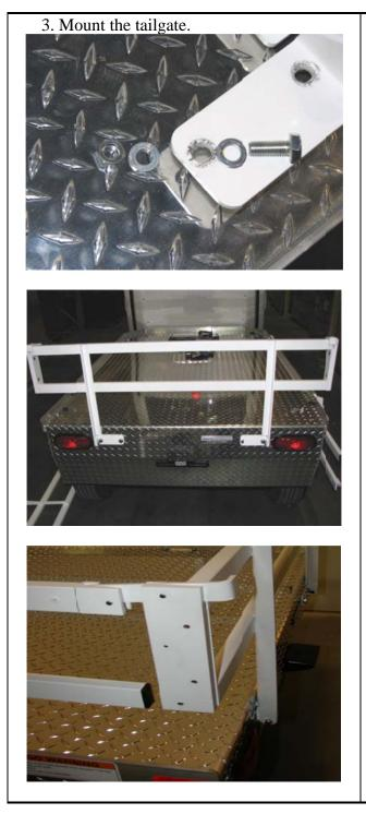
Attach the tailgate to the back of the bed using the existing holes.
