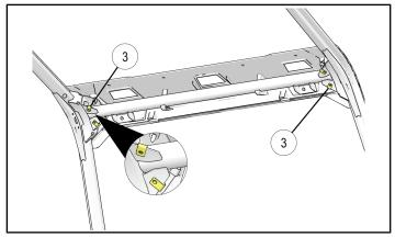
5. Install two nut clips ③ on lower edge of visor panel as shown. Ensure proper orientation.
