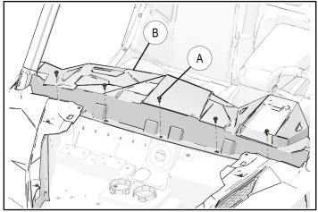
ii. Slide upper dash panel (B) to rear, disengaging eight spring clips (C) retaining upper dash panel to main dash panel (D) as shown.
