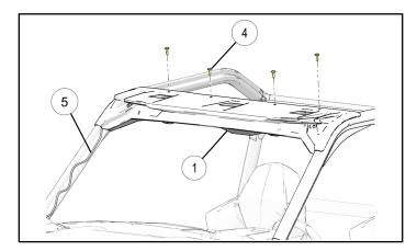
8. Loosely install four screws ② through LH and RH sides of overhead audio ① into previously installed nut clips ③ as shown.
