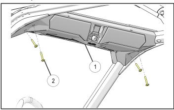
9. Loosely install two screws ④ through lower surface of overhead audio ① into previously installed nut clips ③ as shown.
