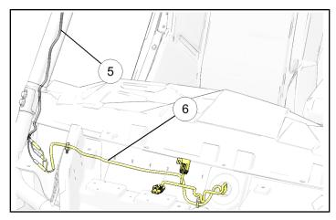
b. Connect three dash harness (6) bullet connectors to corresponding ROPS harness (5) bullet connectors.
