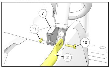
d. Loosely install left frame ② to front bumper using one screw ② as shown.
