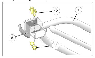
5. Install two LOCK and RIDE® expansion anchors 4 to removable rack ① as shown.
