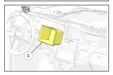
Drill out one accessory plug (1/4 inch / 6 mm) on forward side of firewall, then install relay/fuse block 1B.
