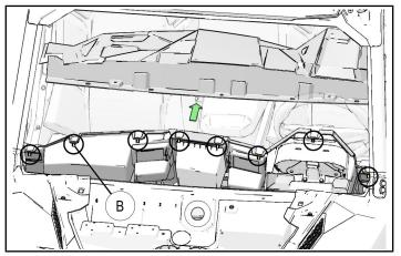
c. Using fingers, remove center storage box ⓒ by pressing top edge of box down, disengaging box locking tabs from main dash panel. Tip box out of dash and remove.
