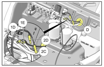
c. Route switch connector 1C on power harness
