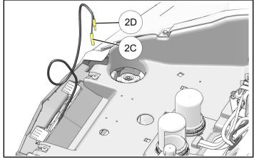
b. Join bullet connectors 1D and 1E on power harness ① to mating bullet connectors 2D and 2C on light harness ②, matching wire colors (red to red, brown to brown).
