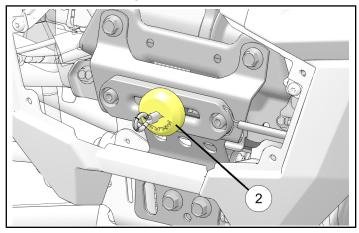
8. Install hook ① to the rope by inserting clevis pin through hook and rope and securing with a cotter nin
