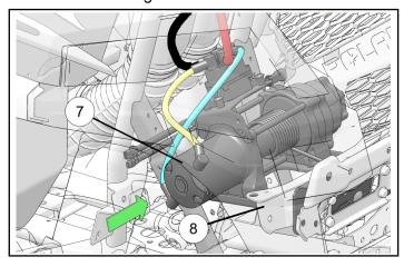
4. Install winch ① to winch mounting bracket ® using four screws ②. Torque fasteners to below specification.
