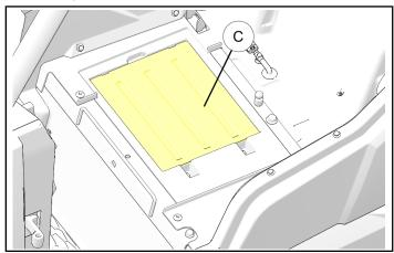
4. Disconnect the black negative cable ① **FIRST** and then red positive cable ⓒ from the battery.
