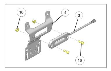
6. Install fairlead mount bracket ④ with autostop fairlead to suspension bracket ⑩ with four bolts ⑤ and nuts ⑰ as shown.
