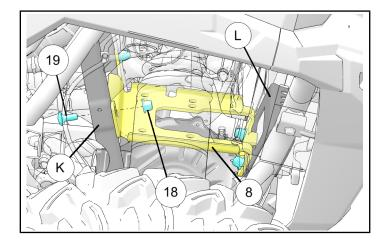
3. Slide and position winch assembly ① onto the winch mounting bracket ⑧ as shown. Ensure mounting holes on winch assembly and mounting brackets are aligned.
