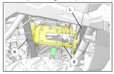
2. Install winch mounting bracket ® onto the front suspension bracket ① and steering bracket ® with four screws ® and lock nuts ® as shown. Torque fasteners to below specification.
