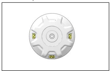
The high gear setting is meant for rapid recovery mode only and should not be used while the rope is under load. To shift into high gear, rotate the gear shifting knob clockwise until the "H" marking shows thru the cutout window on the shift knob. See photo below.
