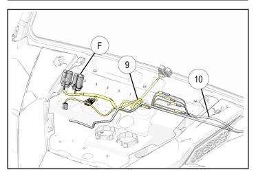
d. On forward side of firewall, drill out two firewall accessory plugs (1/4 inch), then install relays/ circuit breaker (F) as shown.
