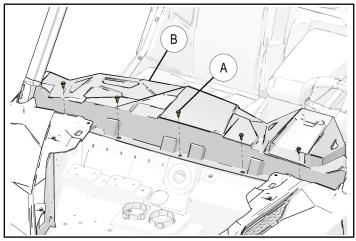
d. Slide upper dash panel (B) to rear, disengaging eight spring clips (C) retaining upper dash panel to main dash panel (D) as shown.
