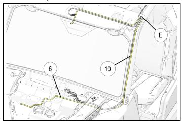
7. Install ROPS harness grommet (E) in ROPS at top of driver side A-pillar.
