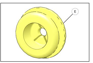
c. Reinstall ROPS harness grommet (E) on ROPS harness <sup>(1)</sup>.
