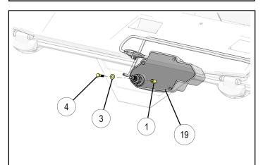
c. Torque motor shaft nut to specification.
