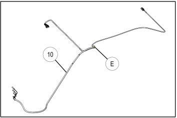
b. Make "X" shaped cut as shown to enlarge interior of grommet (E). Grommet must accommodate harness wiring and washer hose (6).
