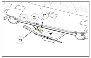
e. Open nut access cover on end of wiper arm <sup>(1)</sup>, then install wiper arm to motor shaft using nut
