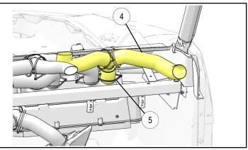
e. Lift main dash panel into position, carefully pulling ducts ②, ③, and ④ through corresponding dash vent openings. Secure outboard ducts to square vents ④ and inboard ducts to rectangular vents ③ with cable ties ⑤, then snap vents into openings as shown.
