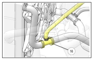
vii. Install hose assembly (1) to "IN" coolant line fitting (2) as shown. Ensure hose is fully seated, then secure with 20 mm hose clamp (1).
