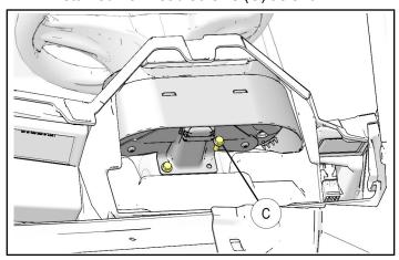
k. Place upper dash panel into position, carefully pulling ducts ② and ④ through corresponding defrost vent openings. Secure ducts to rectangular vents ③ with cable ties ⑤, then snap vents into openings.
