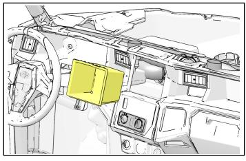
j. Carefully connect instrument cluster electrical harness, then reinstall instrument cluster using retained hex head screws (C) as shown.
