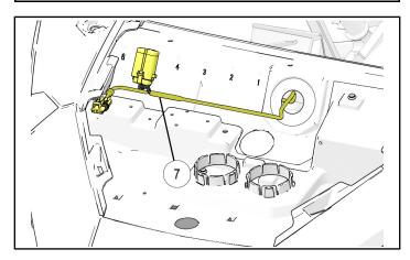
On forward side of firewall, drill out one firewall accessory plug (1/4 inch), then install fuseholder (H) as shown.
