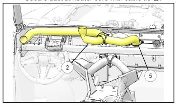
c. Duct ③: Route from heater core to LH/RH inboard dash as shown. Secure duct at heater core with cable tie ⑤.
