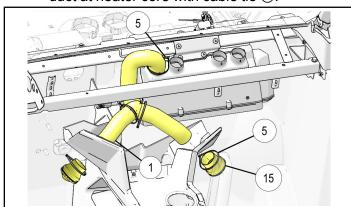
b. Duct ②: Route from heater core to LH outboard dash and LH defrost as shown.
