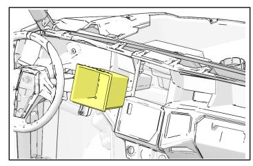
iii. Using fingers, remove center console control panel by disengaging four spring clips (D) as shown, carefully disconnecting electrical harnesses.
