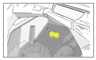
b. Drill three ¼ inch holes in firewall as shown for heater core attach screws ②.
