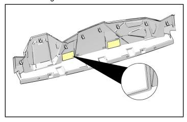
Main dash panel: Cut two rectangular vent openings and two square vent openings on INSIDE EDGE of recessed markings as shown.
