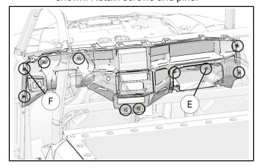
v. Grasp LH center console side panel, then carefully pull panel outboard and downward to detach tabs at location (F1) and (F2) as shown. Repeat for RH side panel.
