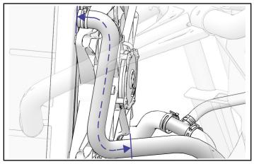
ii. Position hose assembly (1) tee at mark and route opposite end to heater core RH/OUTBOARD coolant line fitting. Ensure routing will prevent chafing against vehicle components or contact with moving parts, taking into consideration suspension travel and steering operation.
