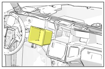
iii. Using fingers, remove center control panel by disengaging four spring clips **D**.
