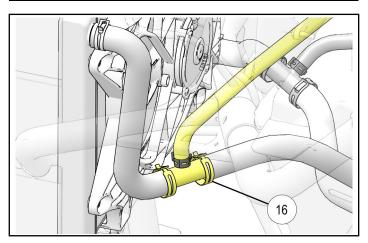
vii. Install hose assembly (1) to "IN" coolant line fitting (2). Ensure hose is fully seated, then secure with 20 mm hose clamp (1).
