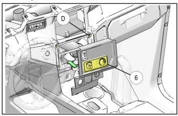
i. Reinstall center storage box by hooking lower edge of box in dash opening, then tip upper edge of box into dash until locking tabs snap into dash panel.
