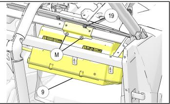
e. Secure front of heater core to firewall using three each screws (2) and washers (2). Tighten screws.
