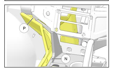
vi. Remove main dash panel, carefully disconnecting electrical harnesses and three lower interior lights <sup>(G)</sup>.
