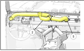
c. Duct ③: Route from heater core to LH/RH inboard dash. Secure duct at heater core with cable tie ⑤.
