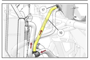
viii.Remove pinch-off pliers from both sides of tee, and from RETURN/COLD hose assembly.
