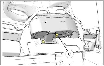
k. Place upper dash panel into position, carefully pulling ducts (2) and (4) through corresponding defrost vent openings. Secure ducts to rectangular vents (13) with cable ties (5), then snap vents into openings.
