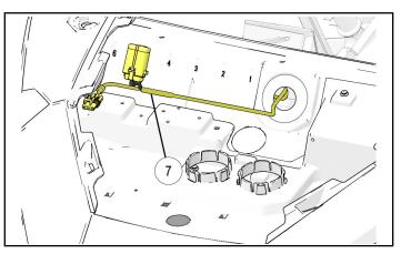
b. Drill out one accessory plug (1/4 inch / 6 mm) on under-hood liner, then install relay/fuse block ⊕ using attached fir tree clip.
