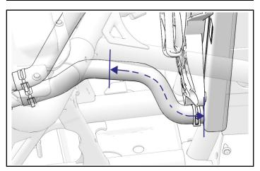
ii. Position hose assembly (10) tee at mark and route opposite end to heater core LH/INBOARD coolant line fitting. Ensure routing will prevent chafing against vehicle components or contact with moving parts, taking into consideration suspension travel and steering operation.
