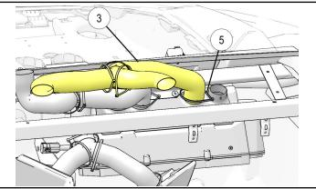
d. Duct ④: Route from heater core to RH outboard dash and RH defrost. Secure duct at heater core with cable tie ⑤.
