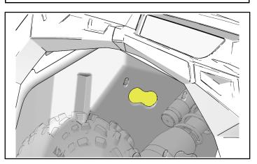
b. Drill three 5/16 inch (8 mm) holes in firewall for heater core mounting screws 2.
