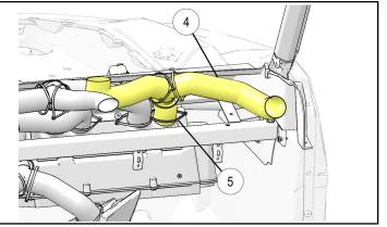
e. Lift main dash panel into position, carefully pulling ducts (2), (3), and (4) through corresponding dash vent openings. Use cable ties (5) to secure outboard ducts to square vents (4) and inboard ducts to rectangular vents (3). Snap vents into openings.
