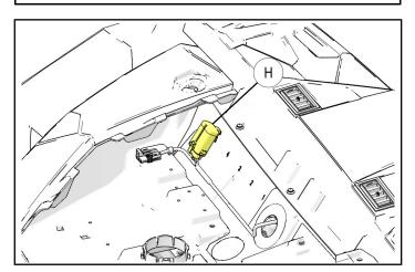
c. Route main heater harness switch panel connectors rearward towards center control panel.
