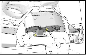
ii. Using fingers, remove center storage box by pressing top edge of box down, disengaging box locking tabs from main dash panel. Tip box out of dash and remove.
