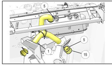
b. Duct ②: Route from heater core to LH outboard dash and LH defrost. Secure duct at heater core with cable tie ⑤.
