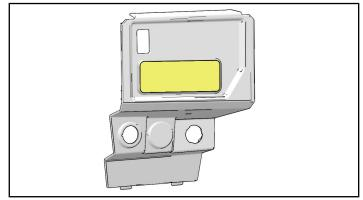
b. Orient switch panel (6) so blower control is on LH side and temperature control is on RH side, then install into opening until tabs lock in place.
