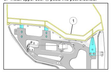
6. With door closed, adjust upper and lower doors as required to fit vehicle opening, then tighten all screws ④. Torque two hinge screws ⑤ to specification.
