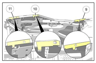
Carefully drill 1/2 inch (13 mm) hole at each marked location.
