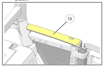
b. Carefully drill 1/2 inch (13 mm) hole at each marked location.
