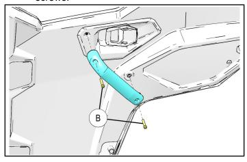
b. Remove two hinge access covers © by carefully detaching upper and lower locking tabs from inner door panel as shown.
