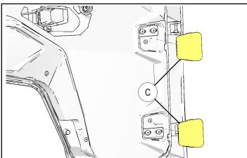
c. Remove six screws (1) and one screw (1) securing inner door panel to frame, then remove panel. Retain screws.
