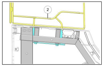
5. Reinstall inner door panel using only FOUR Retained screws (a). Do not reinstall screw (b) at this time.
