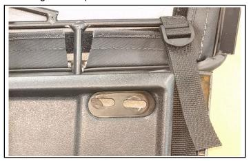
7. Install pull strap ② to upper door ② by wrapping each end of strap around door frame, then snapping ends together as shown.
