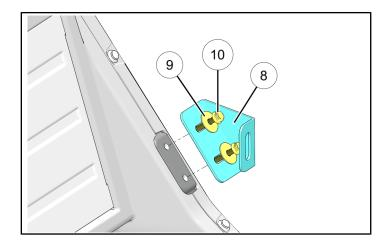
b. Install striker pin ① and conical spring washer
