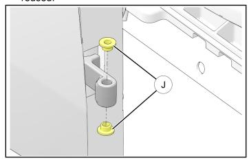
3. Insert new bushing **(6)** TOP-DOWN into all vehicle-side hinges.
