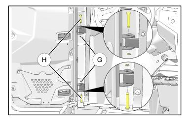
3. Push door inwards while attempting to center door in ROPS/chassis opening. Hold door in place, then observe gap between door assembly ① and ROPS/chassis (around entire perimeter of door).
