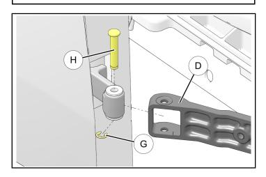
2. Remove upper and lower hinge pin bushings ① from all vehicle-side hinges. Bushings will not be reused.
