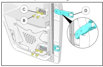
2. Position new door ① so door-side hinge pin holes align with vehicle-side hinge pin holes.
