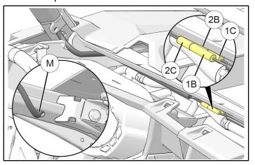
b. Join bullet connectors 2B and 2C to mating bullet connectors 1C and 1B on dash harness
