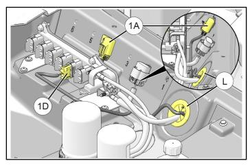
b. Drill out one accessory plug (1/4 inch / 6 mm) on forward side of firewall, then install fuse block 1A.
