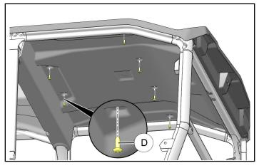
iii. Carefully pull LH and RH edges of liner (E) down from between ROPS and roof seal, then remove rear edge of liner from above C-pillar cross-member. Set liner aside.
