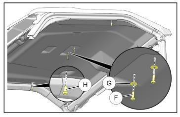
ii. If overhead sound bar is installed, proceed to next step iii. Otherwise remove six screws ①. Retain hardware.
