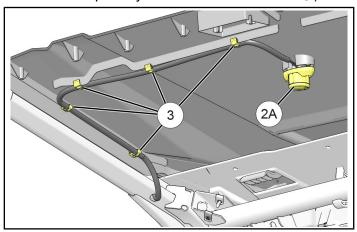
ii. Provide adequate harness slack to allow light base to easily pass through cutout in roof liner (if applicable; see previous Step 4), then secure harness to roof using five edge clips ③.
