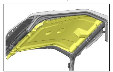
4. Cut dome light opening (§) in applicable liner along **INSIDE EDGE** of recessed marking.
