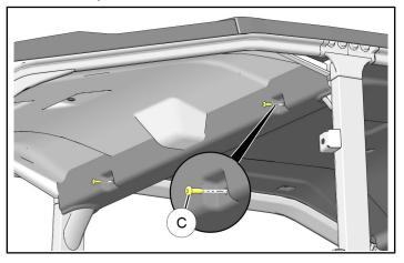
ii. Remove six screws ①, two on rear side of B-pillar cross-member, and four near center of liner. Retain hardware.
