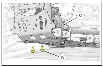
4. Align plow mount ① to bracket (D) and install bolts ⑩ with flat washers ① from front of vehicle and four nuts ④ without washers at rear. Do not tighten bolts at this time.
