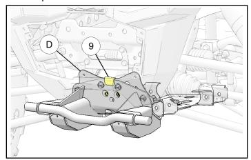
7. Tighten four front bolts (1) to following specification.
