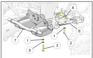
6. If you are not installing a front bumper at this time, set this nut plate (9) aside for possible future use. If you are installing a front bumper, install nut plate in position as shown to allow installation of upper bumper bolts in this location.
