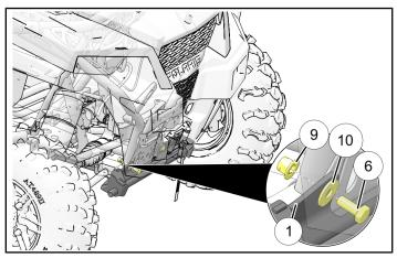
Be sure to place one of the large flat washers (1) on each front mounting bolt (6) then insert the bolts from the front through the mount plate and frame. Start the locking nut (9) by hand on the back side of each bolt to hold into place. DO NOT TIGHTEN at this time.
