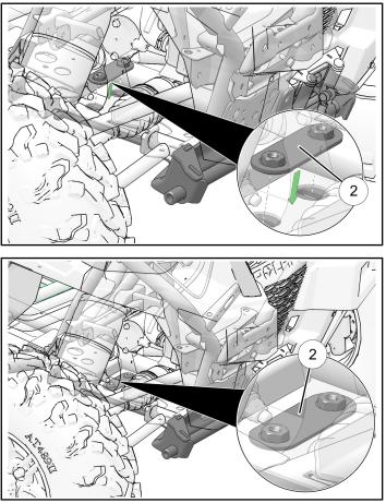
4. Lift rear of mounting plate ① up against the lower portion of the frame and start rear mounting bolts
