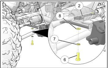
5. Torque front fasteners (9) to specification provided.
