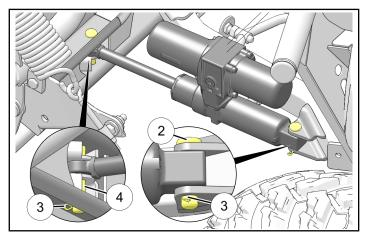
Join connector from angle cylinder ① to mating TILT connector from Plow Controller Kit (PN 2883247 or equivalent, sold separately).
