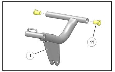
Install upper end of lift arm ① to pushframe brackets using bolt ② and nut ⑦. Tighten nut until play is removed, but not so tight as to prevent lift arm from pivoting freely on bolt.
