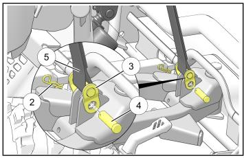
10. Join connector from lift cylinder (1) to mating LIFT connector from Plow Controller Kit (sold separately). Ensure harness routing will prevent binding, as well as contact with sharp edges or moving parts, THROUGHOUT THE FULL RANGE of cylinder travel.
