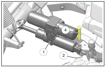
Join connector from angle cylinder ① to mating TILT connector from Plow Controller Kit (PN 2883391 or equivalent, sold separately).
