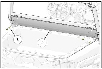
c. Using extension panel (2) as template, mark five holes in existing vehicle close-off panel.
