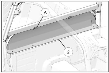
b. Pivot extension panel (2) forward into ROPS, then loosely install four screws (8) through panel into ROPS.
