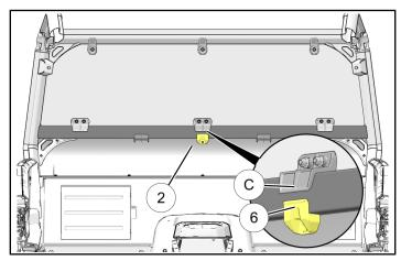
b. Drill 1/4 inch (6 mm) hole through close-off extension panel (2) at marked location.
