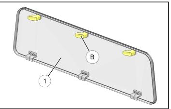
b. Install rear panel ① by inserting three lower brackets ⓒ into ROPS cross-member. Pivot panel forward into ROPS, then rotate handles
