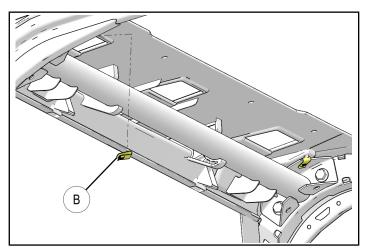
4. Install nut clips (4) to brackets (3) as shown.
