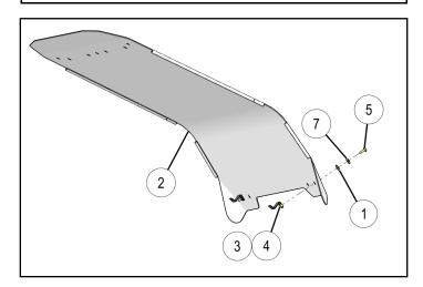
6. Position roof on ROPS, aligning front fastener holes with nut clips (B) or ④.
