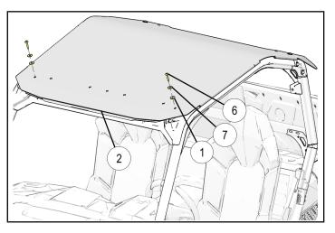
8. Rotate brackets ③ to engage rear ROPS as shown.
