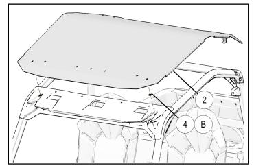
7. Loosely install screw 6 through steel washer ①, rubber washer ①, roof ②, and visor panel into nut clip (B) or ④ as shown. Repeat for opposite side.
