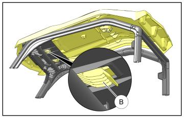
4. Slide roof panel rearward until hooks (B) lock into ROPS visor, then press rear edge of roof panel down until flange (C) locks into B-pillar cross-member.
