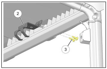
6. Secure front of roof panel to ROPS visor using two screws (1).
