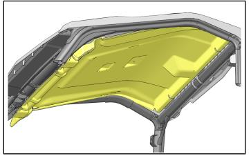
Loosely secure front of roof liner to ROPS bracket and roof using three screws ①. Repeat for RH side.
