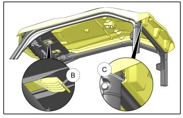
5. Secure rear of roof panel to B-pillar cross-member using bracket (2) and two screws (3).
