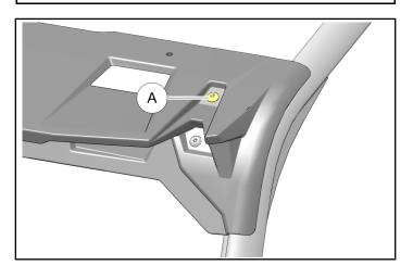
3. Lay roof panel ① on top of ROPS, inserting three hooks ⑧ through openings in ROPS visor.
