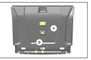
2. Install three clip nuts (8): two on A-pillar crossmember mounting bracket, and one on visor. Repeat for RH side.
