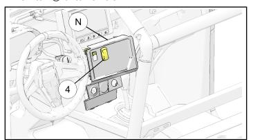
16. Connect main wire harness connection to winch contactor as shown.
