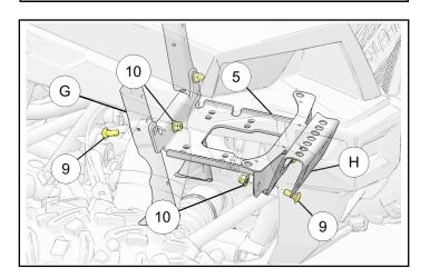
6. Slide winch ③ from passenger side as shown onto winch mounting bracket.
