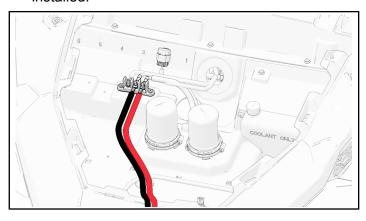
13. Remove control console panel (N) by inserting screwdriver at bottom and pulling control panel outside as shown. Remove one of the rectangular knockout holes. Locate switch connector from main wire harness.
