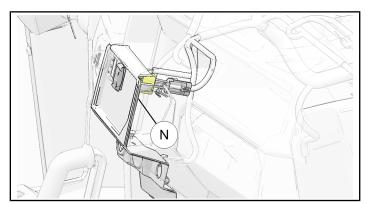
15. Reinstall control console panel (N) with winch switch (4) onto vehicle.
