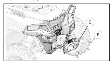
4. Slide winch mounting bracket ⑤ into position from the passenger side as shown.
