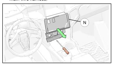
14. Install winch switch ④ onto the control console panel (N). Push switch into hole to seat. Connect switch to corresponding connector on main wire harness as shown.
