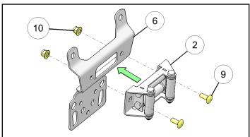
9. Install front plate bracket with roller fairlead as subassembly onto the vehicle with four bolts ① and nuts ①.
