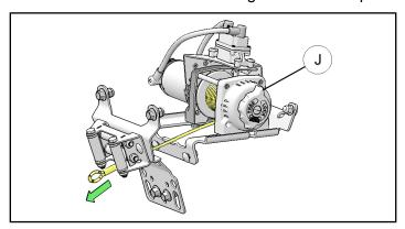
11. Attach hook ① to the rope by inserting clip through it.
