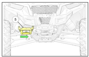
5. Install winch mounting bracket ⑤ onto the front suspension bracket (H) and steering brackets (G) with four screws ⑨ and lock nuts ⑩. Torque to below specification.
