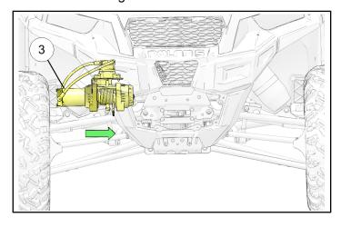
Install winch ③ onto the winch mounting bracket
