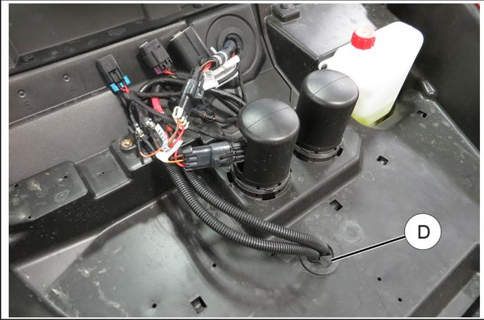
8. Secure winch contactor connector using fir tree clip.
