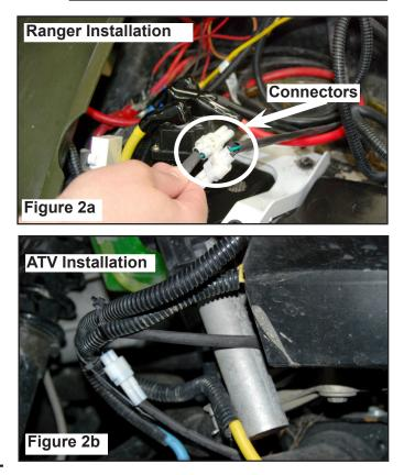
Disconnect the remote control from the winch contactor, and plug those two connectors into the corresponding connectors on the control harness. Figure 2.
