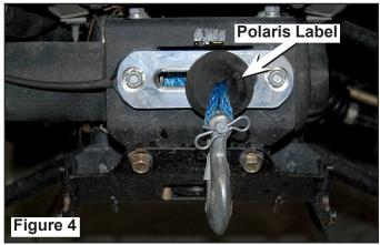
5. Before use, confirm the proper function of the AutoStop by turning on the winch and spooling it in. The rubber stop should get close to the fairlead and the winch should turn off automatically. If it does not, check that all connections are made properly and that the rubber stop is facing with the "POLARIS" side facing outward and retest.
