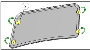
3. Install windshield ① into ROPS, then turn handles② to locked position (perpendicular to sides of windshield) as shown.
