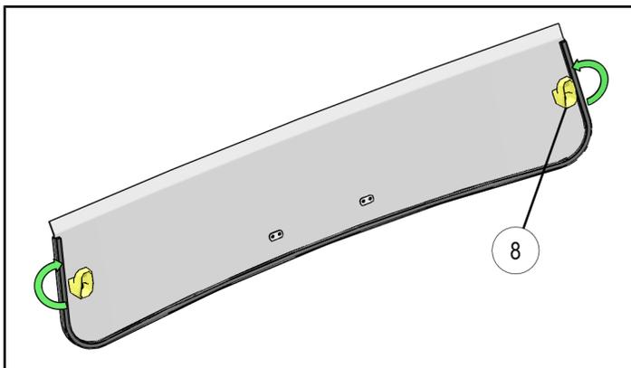
4. Install windshield ⑤ by inserting brackets ⑥ into newly cut slots (E) as shown. Pivot windshield into ROPS, then turn handles ⑧ to locked position (perpendicular to sides of windshield) as shown.
