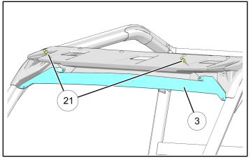
c. Using upper trim panel ③ as template, mark and drill two 5/16 inch holes through visor, then secure using two push pin rivets ④ as shown.
