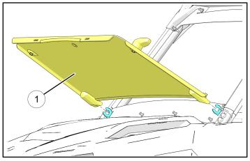
c. Tip windshield assembly ① up as shown, then rotate both handles © 1/4 turn to lock windshield to A-pillars. Adjust brackets ⑫ and ③ as required to ensure windshield assembly is centered in ROPS opening.
