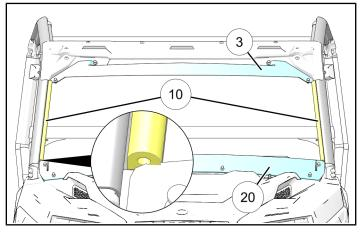
b. Position windshield assembly ① as shown, then insert into hinge assemblies.
