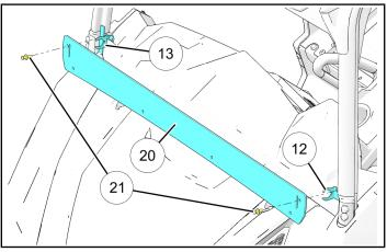
f. Using lower trim panel (2) as template, mark and drill four 5/16 inch holes through upper dash panel. Starting from middle of lower trim panel, secure using four push pin rivets (2) as shown.
